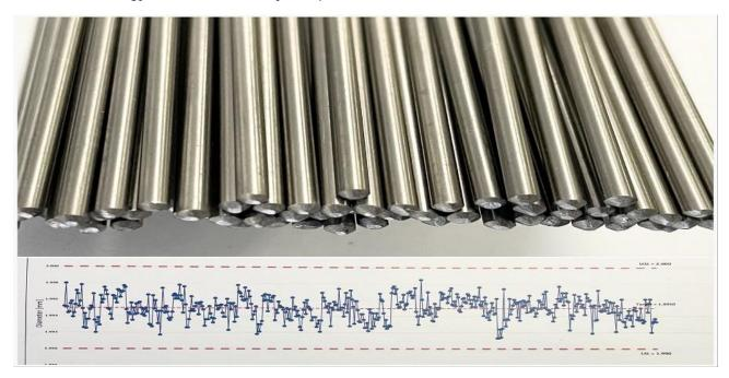
Lower tool wear, reproducible, high-precision parts and minimal downtimes, especially in unmanned production, increase efficiency despite higher material costs and ultimately reduce unit costs. Signer Titanium also offers the service of measuring and recording round bars up to 5 mm in diameter using an optical micrometer. Individual bars or entire batches can be documented and statistically evaluated with several measurements per bar, thus enabling the process capability to be assessed.
